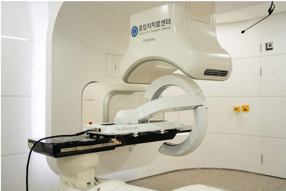
Figure 3: Terapet's Qualyscan in action at Yonsei Cancer Center (These pre-clinical tests were carried out with a goal to demonstrate the feasibility of using Terapet's technology in a heavy ion setting, involving device installation, stress-testing and performance characterization.)
